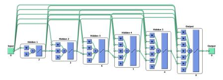
Cascade forward nets are available in the Deep Learning Toolbox in Matlab and can be used together with the System Identification Toolbox to facilitate comparisons with other model types
