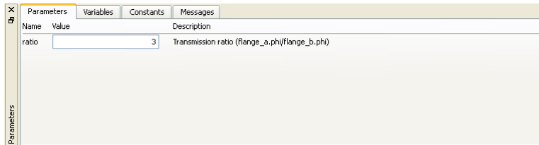
Figure 3-11: Editing the transmission ratio of a ideal gear component in the model editor.
