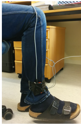
Figure 2: Experimental setup with IMU mounted close to the user's foot.
