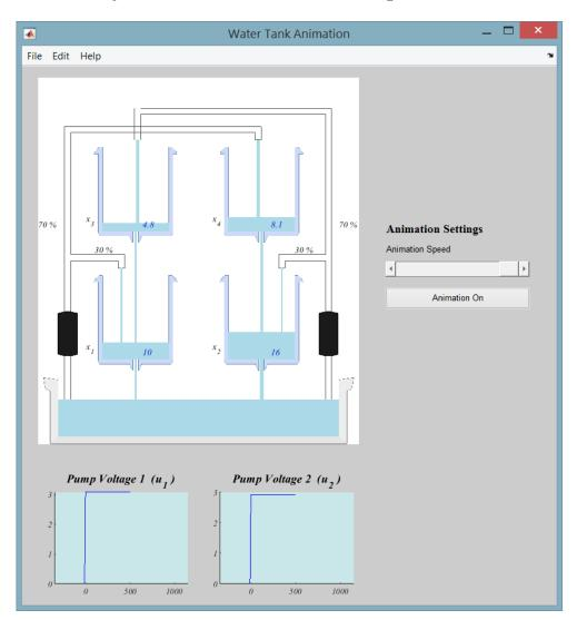
The simulation model also has an animation that illustrates the behavior of the tank system. The animation is shown in figure 2.
