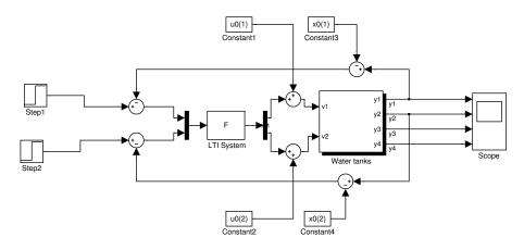
Figur 3: Typical Simulink model with a multivariable controller working with deviations from a working-point.
