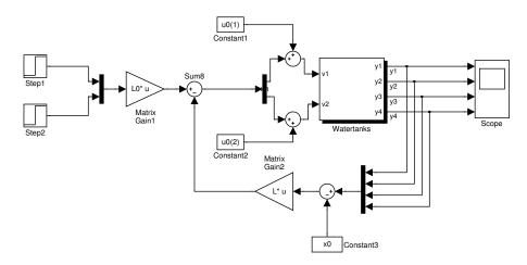
Figur 4: State feedback around stationary point
