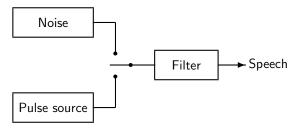
The speech is seen as a sequence of either voiced or unvoiced sounds. The voiced sounds are modelled as a filtered pulse train, while the unvoiced sounds are modelled as filtered white noise.
