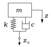
The car is traveling at 70 km/h on a sinusoidal road with wavelength 15 m and amplitude of 10 mm. Determine the maximum force between tire and ground.
