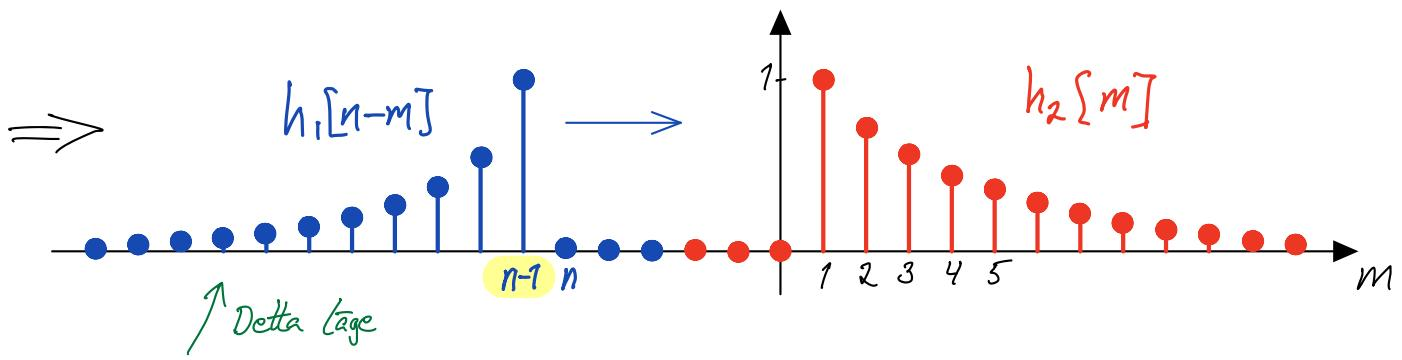
$$\bullet n-1 < 1 \text{ dvs. } \underline{n \geq 2} \Rightarrow h_1[n-m]h_2[m] = 0 \Rightarrow \underline{h[n] = 0}$$
